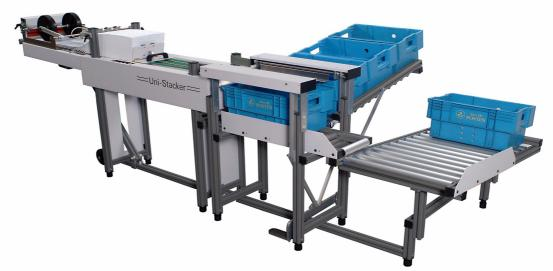
Uni-Stacker is a receiving system that, thanks to it's vertically installed input device and choice receiving packet which can change for driving from left, right or straight forwards can be adjusted to most of the inserting systems.
